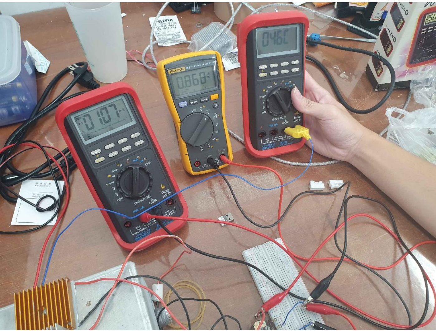
Figure 6. Experimental Setup for Measuring Loaded Voltage and Current.
